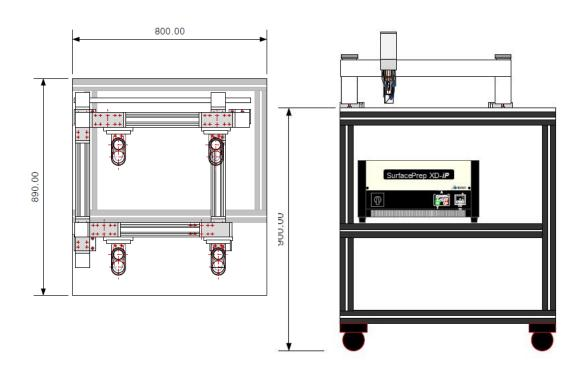
SurfacePrep XD systems require either compressed air supply from a clean, dry source or bottled gas such as oxygen, nitrogen, argon or CO2. "Welding Grade A" purity is acceptable ultra high purity not required.
