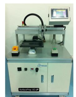
Works on both conductive and non-conductive materials. Low temperature plasma is safe on sensitive polymers, thin films and glass. Treat stainless steel, Ti, NiTi, Au and other metals as well as these polymers:
